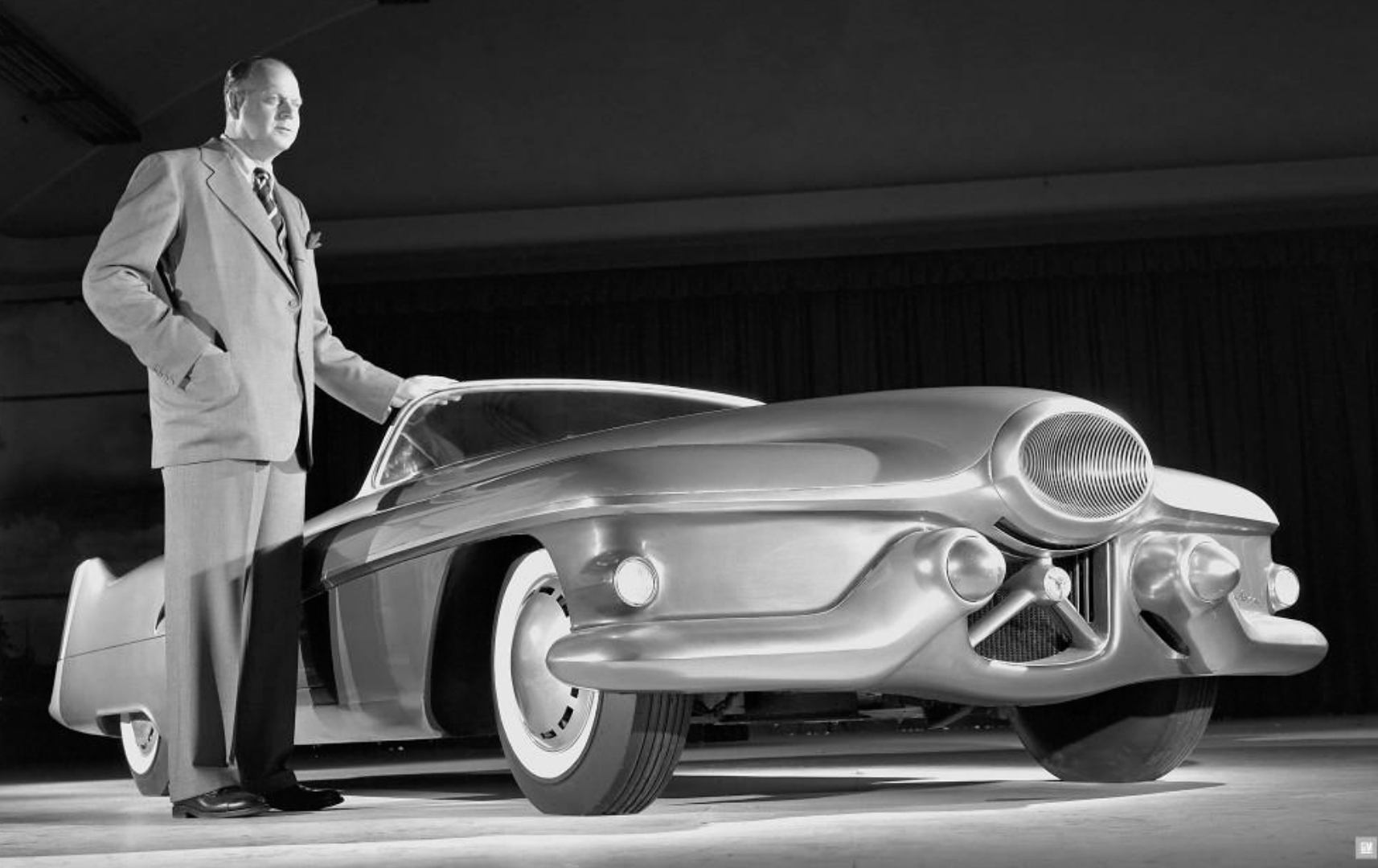
Harley Earl introduced clay modeling to automobile design. Here he stands next to a wood and clay model of the 1951 Buick LeSabre concept car. Courtesy General Motors.
