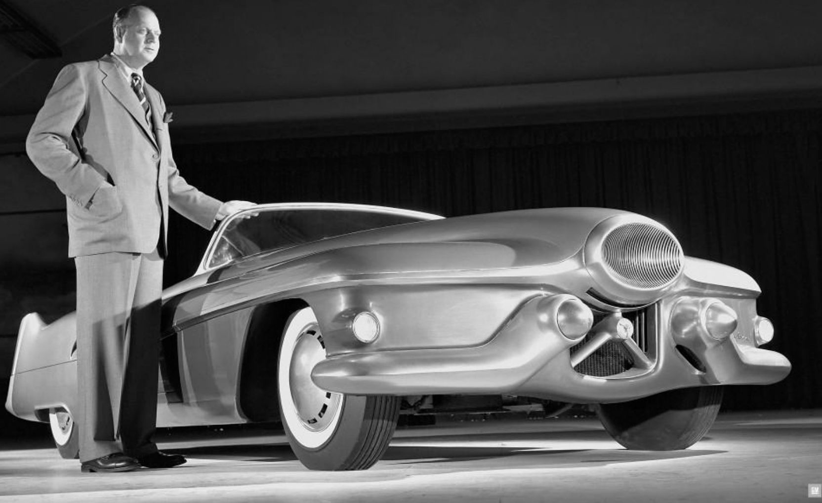
Harley Earl introduced clay modeling to automobile design. Here he stands next to a wood and clay model of the 1951 Buick LeSabre concept car. Courtesy General Motors.
