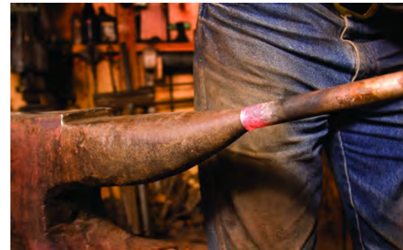
Figure 8.32. Flare the top of the socket.
