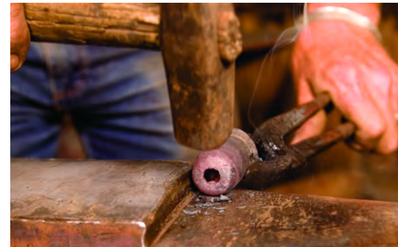
Figure 8.33. Close the base of the socket.
