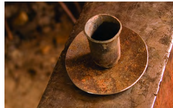
Figure 8.34. Socket and drip pan are ready to be riveted to the base.
